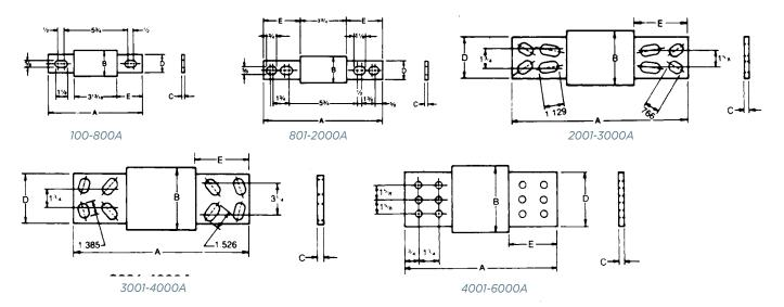
Safety Note: Class L fuses are dimensioned for one-way interchangeability. A Class L fuse of any lower ampere rating can be substituted for a given Class L fuse.
