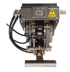
Current collector devices are used by Metro to collect the energy from the third rail to energize the Electrical Multiple Unit installed in the trailers.
