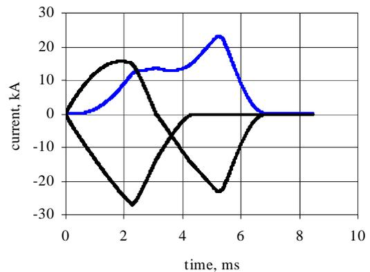
Figure 17. Currents for arcing fault with fuses
