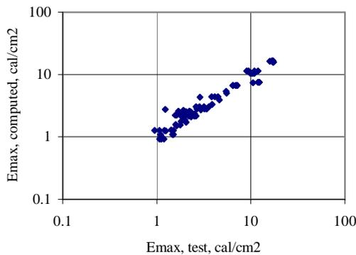
Figure 12. Predicted incident energy density, all open tests
