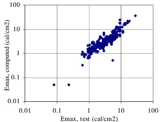
Figure 14. Time domain model prediction compared with test
