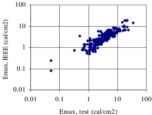
Figure 15. IEEE formula prediction compared with test
