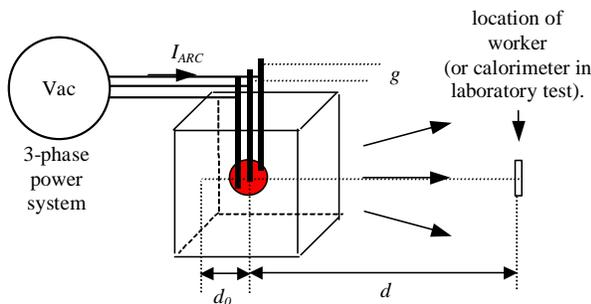
Figure 1. Arc flash in an open box
