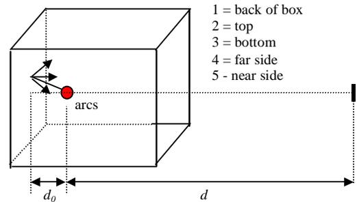
Figure 13. Box geometry for calculation of reflections
