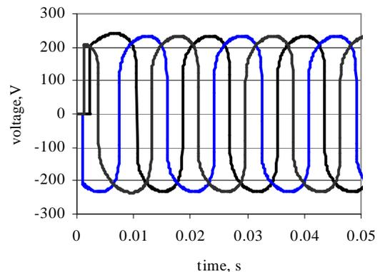
Figure 6. Computed fault arc voltage transients
