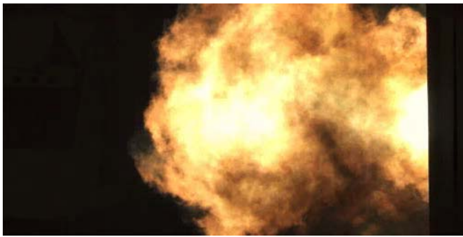
Figure 4. Arcing with horizontal electrodes at back of box.
