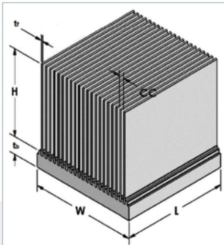
Fig. 3. Heat sink Dimensions Sketch
