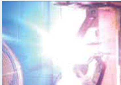
Figure 4: Case rupture of MOV during abnormal overvoltage test.
