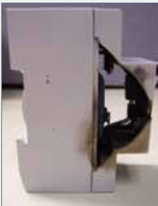
Figure 3: TVSS damage due to abnormal overvoltage test.
