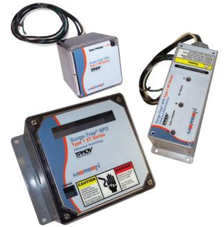
Surge-Trap Type 1 X-Series SPDs feature a NEMA 4X enclosure and can be installed line-side or load-side of the main disconnect. They have a 20kA nominal discharge current and 200kA SCCR rating (most models) and are suited for system voltages from 120V to 600V.
