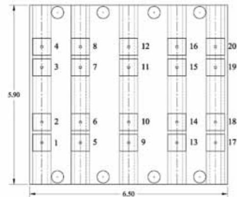
Fig. 4. Thermocouple layout and chip location on the heater block.
