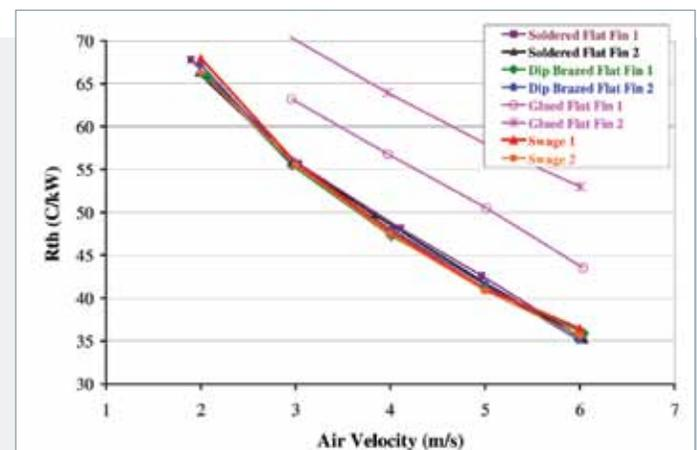
Fig. 8. Test results for all samples.
