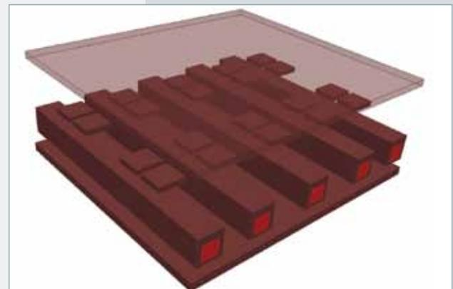
Fig. 5. IGBT replica heater block
