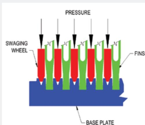
Fig. 1. Diagram of the swaging process of bonding the fins to the baseplate
