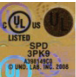
Figure 3: A picture of a holographic label from a UL 1449 3 rd edition device. Please note the SPD wording, which is accepted in today's industry.
