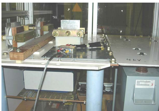
Fig. 5. General overview of the high di/dt test bench at Mersen's Saint-Bonnet de Mure lab (France)
