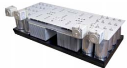
Figure 8: Power electronics assembly with the integrated architecture approach
